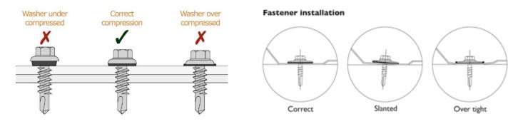
TIP: Make sure fixings are not over tightened as this can burn off the soft neoprene pad under the washer
